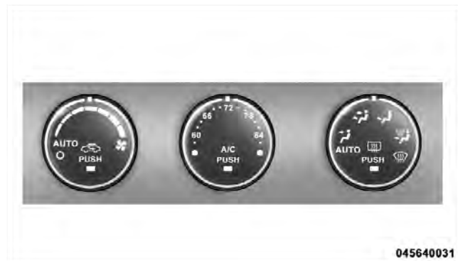
Automatic Temperature Control
